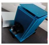
RICX300 series light source has high output from UV to NIR, RICX300-F focus on simulated sunlight of visible light; RICX300-UV has strong continuous output within 200-400nm and focus on applications of high UV requirements.
